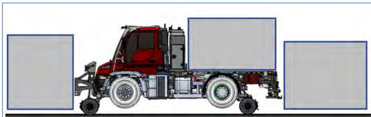
Equipment carrier with various attachment options for modules and equipment
